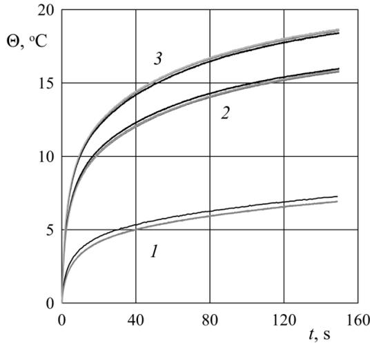
**Fig. 3.** Temperature data for experiments with different materials: 1 – AISI 304, 2 – Ti64, 3 – Ti64 processed.
