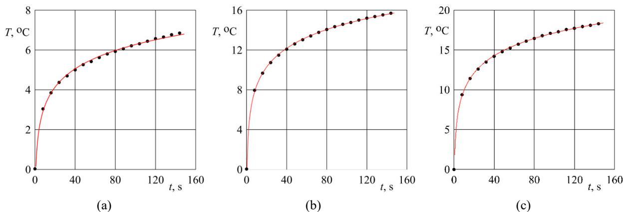
**Fig. 4.** Comparison of the experimental points (black, every two hundredth point is shown) with theoretical solution (red line): (a) AISI 304, (b) Ti64, (c) Ti64 processed.
